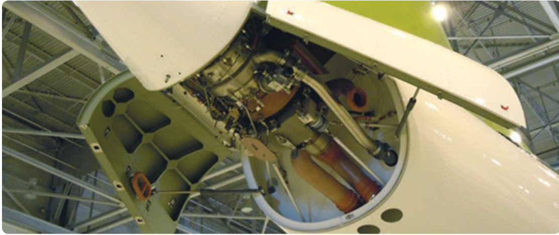
Figure 18-5. typical empennage/tail cone APU installation.
