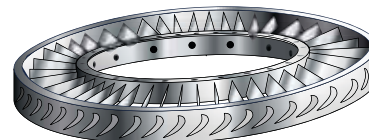
B. Turbine nozzle vane assembly with welded vanes.
