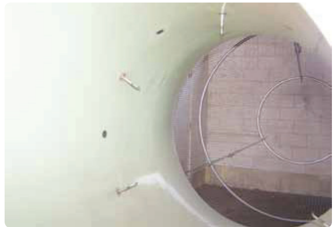
Figure 3-9. Probes within a bellmouth inlet used to measure intake temperature and pressure.
