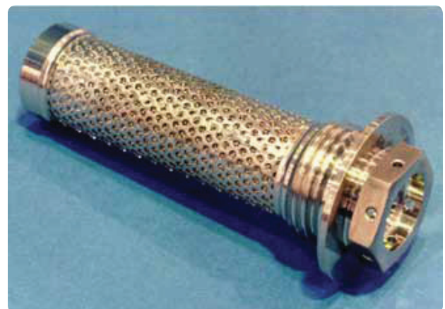
Figure 10-6. Last-chance filter before spray nozzle.
