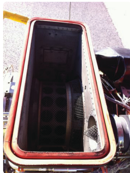
Figure 18-1. APU intake note FOD/ice screen around impeller.
