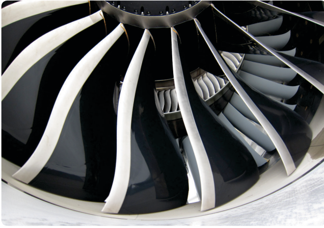
Figure 3-2. Inlet fan blades and guide vanes (inner circle) on a GENx engine.
