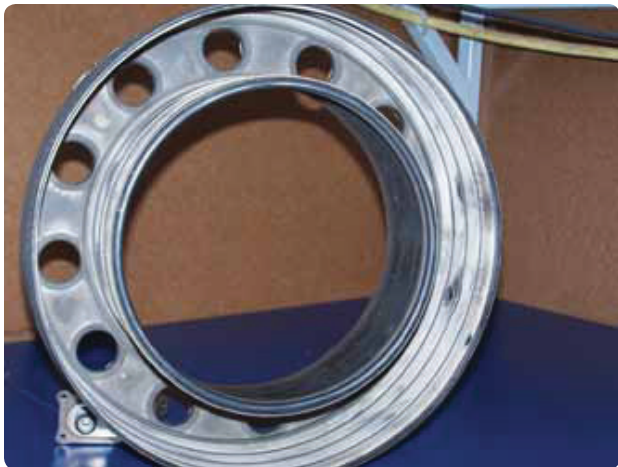
Figure 5-7. Annular combustion with chamber ceramic coating.
