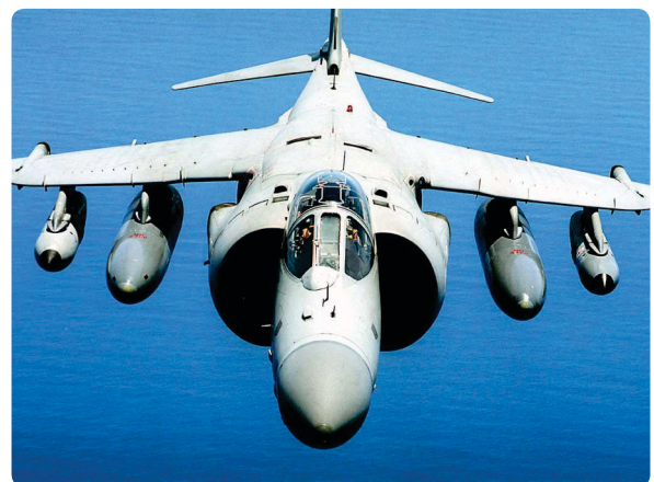
Figure 3-3. An example of a divided-entrance duct.
