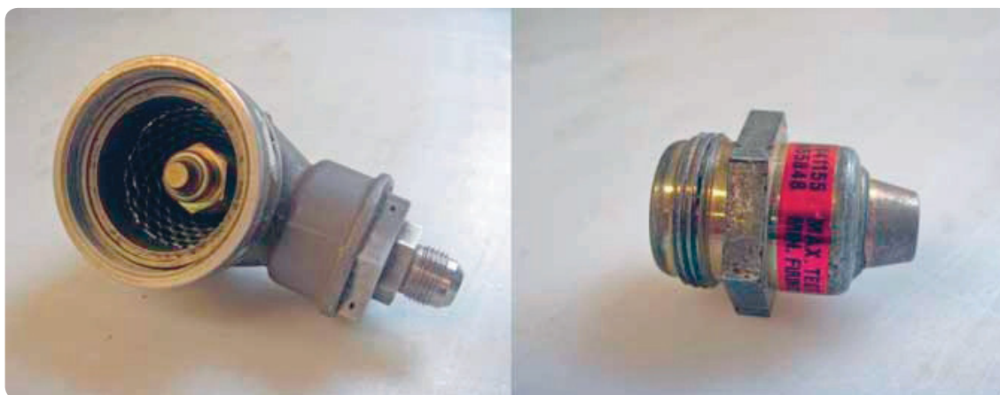
Figure 20-10. Discharge valve and cartridge (squib).
