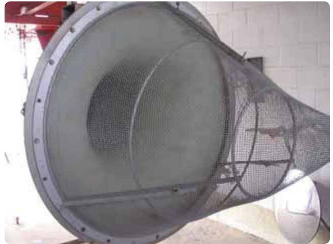
Figure 3-8. A bellmouth inlet used during system tests.
