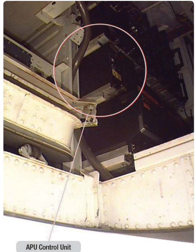
Figure 18-8. APU EEC location in an aircraft's forward avionics bay.
